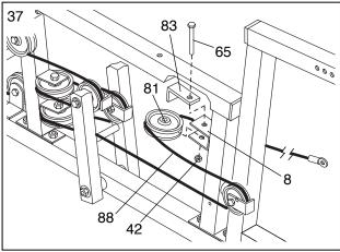
38. Note: The 3 1/2" Pulley (82) used in this step was attached in step 36. It is shown removed for easier part identification.
